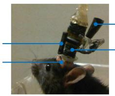
Fig. 76: Headstage connected to a rat.
