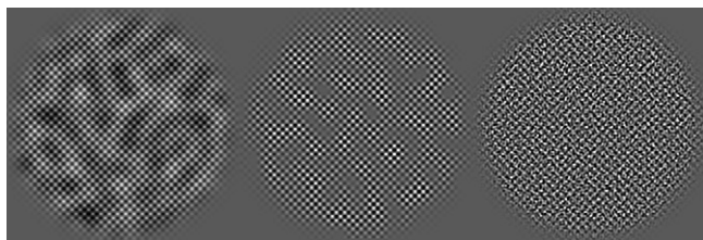
Fig. 5. LM- (left), CM- (center) and carrier-noise (right), all three in the presence of a carrier.
